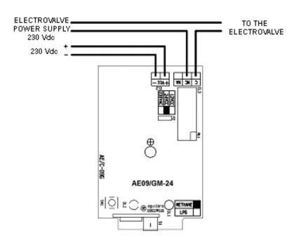
Electrovalves are usually open when being fed. When cutting-off the power supply blocks the gas flow and manual reset is required.
